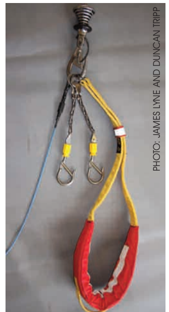
TOP: SAR DOG AND HANDLER LEFT TOP: STATIC DISCHARGER, TWO GRABBITS AND STROP
